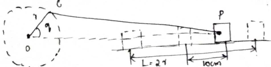
$$\text{Speed of crack} = 420 \text{ rph} \quad \omega = \frac{2\pi N}{60} = \frac{2\pi \times 420}{60} = 43.98 \text{ rad/s}$$
