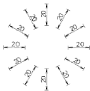
Fig. 4.10 Indicating dimensional values on oblique dimension lines (Method-1).
