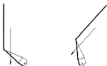
Fig. 3.4 Sketching of vertical and inclined lines.
