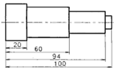
Fig. 4.15 Parallel dimensioning.
