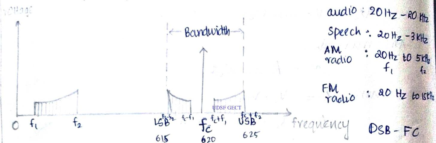
$$\text{Bandwidth} = 2 \times f_2 = 2 \times \text{highest modulating frequency}$$
